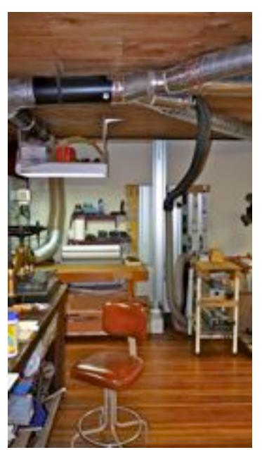
With that set up I can reach about a 25' radius all around the studio and out into the gallery area where the Felder RL-200 dust collector is located. That is really handy to vacuum up any dust that escapes from the DC while I am emptying the bins.
