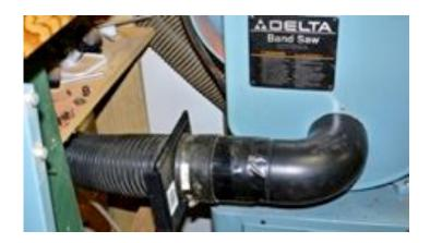
The left most branch services the two band saws, the 17" wide belt sander and the combo machine. Only one of those is in use at any time so the 6" line works just fine servicing those machines.
