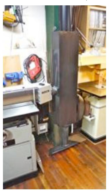
My solution was to build a distribution box that hangs on the wall. The 6" trunk line comes in the top. Two 4" blast gates supply the spindle sander along one side of the box. Two blast gates along the other side of the box supply the belt sander and one on the bottom of the distribution box goes to the floor sweep. Since no more than two of these are ever open at the same time, this system works quite well.
