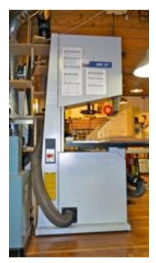
dust was carried in the blade gullets and thrown off elsewhere. To help capture that dust, I again added a 4" port to the lower door.
