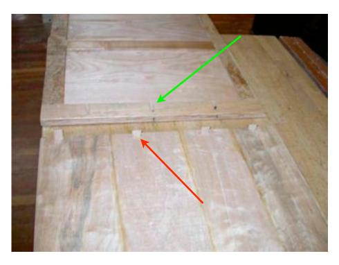
by one or two Domino placed along the thickness of the edge, it is good practice to stack Dominos using multiple sets in the same joint. to side the joint edge closest to the point of force is placed in tension while the side of the joint furthest from the point of force is placed in tension. The shorter the dis-
