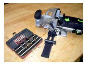
the Domino fence to be exactly 22.5mm to center those on the 45mm thickness of the legs. They must be spot on because those skirts will sit in a dado we will cut in the platform frames and they have to also index into the legs via these Domino M&T joints. I keep a set of metric gauge blocks around just for such purposes. Remember the step block built into the base of the Domino machine? That slides back
