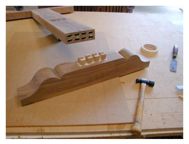
This photo (supplied by Festool) shows one example. The leg to base joint uses eight Dominos stacked in a  $2 \times 4$  array while the leg to stretcher joint uses six Dominos stacked in a  $2 \times 3$  array.
