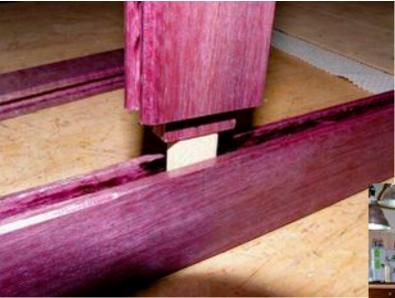
With the back now finished it is time to mate the dovetailed and end mortised rear lower frame rails (which also have the groove that will hold the bottom of the cabinet in place) to the bottom of the back component. Since this is a long
