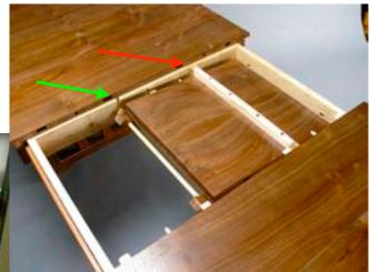
hinge line in the leaf will be exactly in the middle of your table. When the leaf is folded and stored beneath the top plates the hinge side of the leaf must clear the inside edge of the frame. So, the distance from the inside of the frame to the center of the pivot mechanism dovetail slot has to be about 15mm to 20mm
