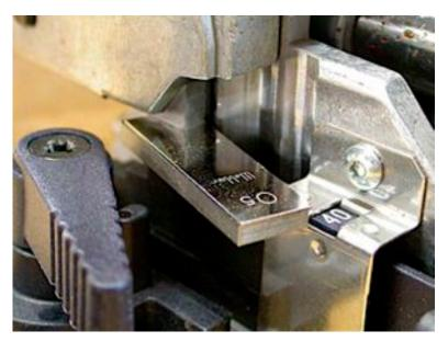
and forth to establish a step that will position the Domino fence up half that amount from the centerline of the cutter. One of those stop block settings is for 40mm thick material and it will position the cutter right in the center, or 20mm up. We need 22.5mm up to center on our 45mm legs, so I placed a 5mm gauge block between the step and the fence to register the fence for a 45mm stock thickness to put the cutter centerline up 22.5mm.
