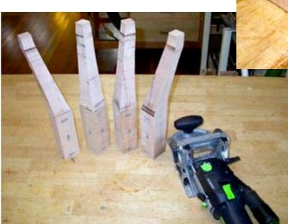
leg we saw before. In this case the legs just flair out in both dimensions so they look right in either mode. In this photo the leg blanks were glued up, a template used to mark the flair, and a band saw used to cut the rough shapes shown here.
