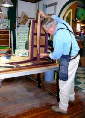
between the two leg stretchers using Domino tenons inserted dry (no glue) into wide mortises cut on the inside of the stretchers and the ends of the shelf. From previous descriptions, aligning these
