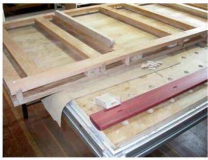
You can see that in the bottom photo. The trim is inverted so I can countersink into the edge that will be against the top.
