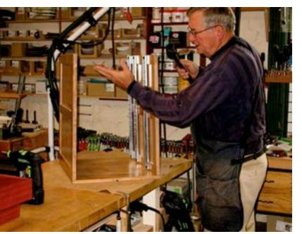
In the lower photo you can see the faux drawer end attached to one side, and below while I am installing the drawer slides. It was easy to build the blood wood top-ofpedestal stand offs using the Domino M&T joint to strengthen the otherwise weak miter joint. It is hard to see in these small photos, but the top of each pedestal is plywood for strength and each is inset into rebates in the sides and backs. The blood wood stand offs attach to those from underneath where the fasteners won't be seen.
