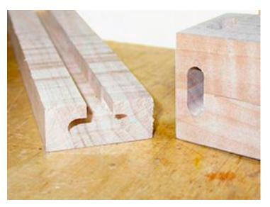
with the end of the work piece and plunge to make the cut. The result is shown on the bottom of the previous page along with one of the legs that it will mate to.
