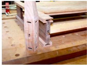
how the vertical M&T joint between the leg and the side skirt will make up as the skirt slides in the dado and onto the leg tenon.
