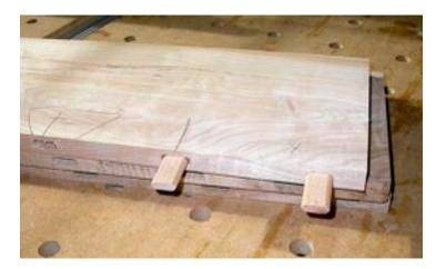
Do that on both boards. Since the spring loaded pins set the horizontal mortise center and the fence sets the vertical mortise slot center, the ends and the faces of the two boards will be perfectly aligned. In the photo above you can see that I mark the end aligned with the spring loaded pin with an "X" mark. That mortise is centered 34mm in from the edge.
