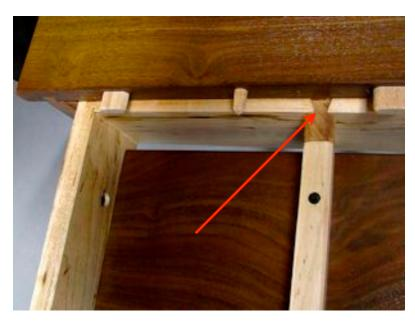
sembly. When everything is square the pivot mechanism (red arrow in this photo) slides in the dovetail groove until it is snug to the underside of the leaf. At that point the leaf is screwed to the pivot mechanism and the dovetails on either side are pinned in place so the pivot point can no longer move.
