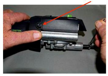
other hand. In the photo above I moved my thumb down so you can see the shaft lock lever (red arrow).
