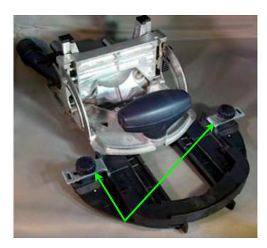
The saddle fence slides onto the fence
