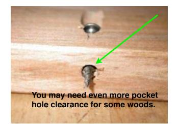
one piece aligned with the face of the other, I am using four Domino M&Ts *without glue* to hold the alignment (red arrow), and pocket hole screws with elongated screw holes (green arrow) to actually hold the two pieces tightly together while still allowing one to slide enough relative to the other....a very handy trick to keep in mind.
