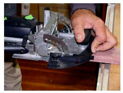
through to the good side of your work pieces. Usually that will mean placing the mortise below the joint center as shown on the previous page and using a short tenon. This is where the 12mm cut depth setting is really handy.
