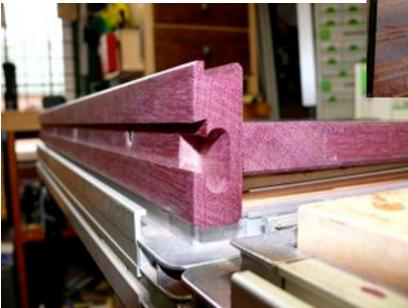
As we assemble we can slide the lower maple curved pieces into the sliding dovetail slot while we insert the Domino tenons to affix the back and the front frame members to the sides we completed earlier.
