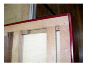
The next step was to provide for the banding across the front. I made work surfaces by Domino M&Ting (is that becoming a verb?) the plywood extending work surface to a side slide that would hold the work surface flush with the underside of the top as shown here.
