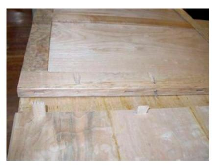
The screw into the tenon prevents the tenon from withdrawing from the unglued mortise in the side stile while it still allows the solid maple pedestal faux drawer open pedestal as these slots are actually quite attractive and will not detract from the look when that open pedestal becomes a bookcase in the future. For the back side of the drawer pedestal that will never be seen from the inside and which
