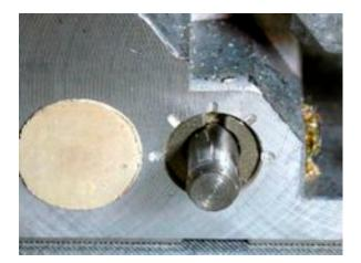
The vertical centerline of the cutter is also marked in several other ways (red arrows) as well: by the "V" cast into the fence base, by the line scribed on the base of the fence (the fixed portion). I placed a rule on the inverted base of the fence for the bottom left photo so you can see the centerline of the cutter lined up
