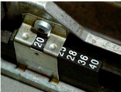
For rapidly setting the fence to common heights above the horizontal centerline of the bit, a stop block (shown in detail above) is provided that slides back and forth to reveal different step heights. The
