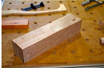
we discussed earlier. Simple to do, just set the height pointer to 25mm and lock the fence as shown in this photo (the Domino body has been removed from the fence so you can more easily see the height setting). Place the Domino fence on the leg surface where you want the mortise and slide it to where the centerline mark aligns with the mark you made on the leg blank, turn on the Domino machine and make the cut.
