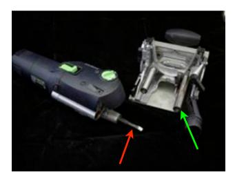
The fence will start to slide off the body as shown in the photos left and above exposing the rotating and oscillating cutter (red arrow).
