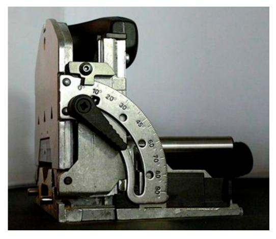
common intermediate settings, or you can simply set the angle with the protractor scale and pointer. The pointer is adjustable so you can calibrate the angles to be dead on.
