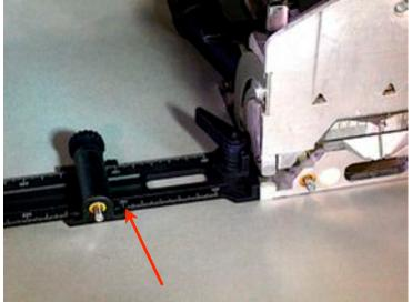
In the photo above the inside edge of the spring loaded pin is set to be 150mm away from the horizontal center of the mortise slot. The red arrows show the alignment scale and pointer.
