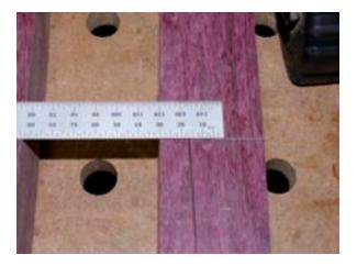
the leg curved you need the cut off piece to get a reference. Be sure to align the cut off pieces in the same place up and down on the leg so the relative saw kerf is the same on all four legs.
