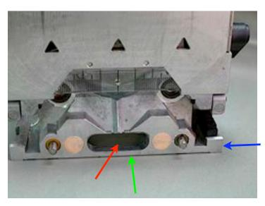
emerges when the body is pushed towards the work piece to make the mortise cut. The cutter centerline is 10mm up from the base of the fence assembly (green arrow above).
