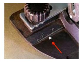
piece? Set the fence to 10mm high and set the two sides of the saddle fence to 25mm as shown above. The resulting mortise will be exactly centered in the end grain no matter which cutter you use or which width setting you select. Neat!
