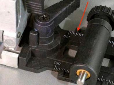
the mortise slot 105mm away from the edge of the work piece that rests against the stop pin.
