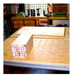
the outline of the square top of the leg on each block and draw an arrow pointing diagnonally out to what will be the outside of the cabrio curved leg.
