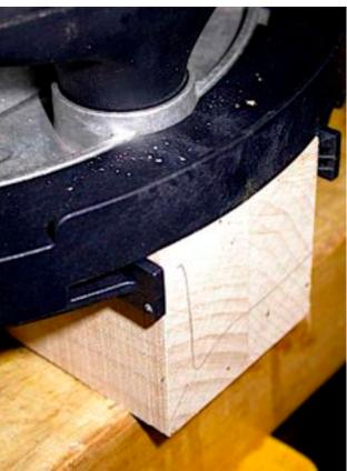
we need three Domino mortises on each of two sides of each of four legs. The upper and lower horizontal mortises will attach the legs to the platform frames while the vertical mortise will attach the skirts to the legs.
