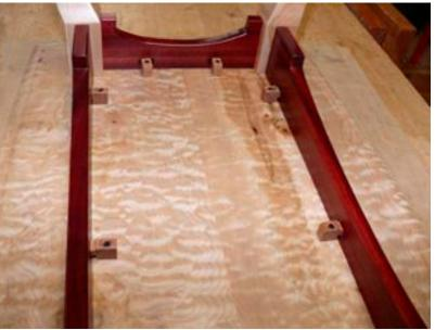
You can also cut these mortises from the top side if you want more bottom of slot to underside of top dimension. Set the Domino fence height to wherever you want the center of the slot. Add on the auxiliary base for stability. Place the fence on the top edge of the skirt with the auxiliary fence held to the inside face of the skirt and make the cuts. Machine tongue blocks to match, screw them down as shown and you are done. Al-most.....
