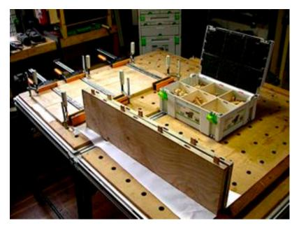
I suggest you always work with the fence on the top or "good" surface of your work pieces so those faces will align even if the two work pieces are not exactly the same thickness.
