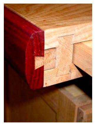
dovetails too close to the edge of the top or the stresses from normal seasonal movement might break off the edges of the dovetail grooves.
