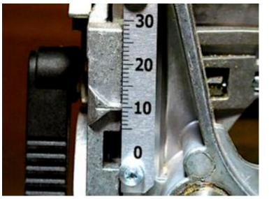
fence sits on the top of a stop block step, positioning it exactly an indicated distance above the horizontal centerline of the cutter.
