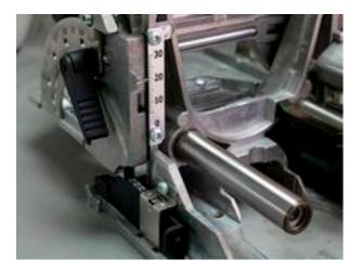
The first adjustment to consider is the height the fence is above the *horizontal centerline* of the cutter. That is shown by a scale and pointer. In the close up photo below the fence is set to be exactly 10mm above the centerline of the cutter. A lock lever secures the fence at the desired height. The fence moves up and down on machined ways so it remains exactly parallel with the cutter at all heights.
