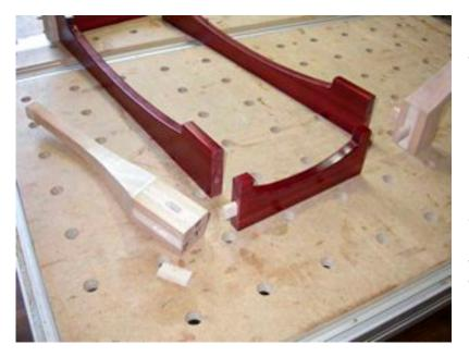
It is easy to make a tongue block with the base of the tongue up slightly less than 7mm from stock that is 12mm thick. That will present a 5mm tongue to insert into the 6mm slot cut on the inside of the skirts. By keeping the bottom of the tongue a bit less than 7mm, when you screw that block to the underside of the table top the tongue will press the skirt firmly to the top while still allowing it to move with normal seasonal changes in humiditv.
