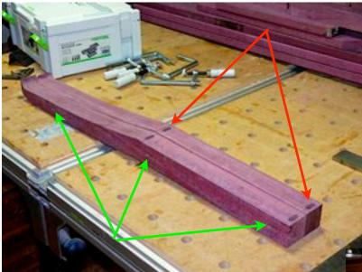
As before, let's start with the legs. Glue up stock to make four blanks. In this case the legs flair out side to side, but not front to back. Construction is the same, but we only need to scribe our template on one face, not both faces as is the case with cabrio legs.
