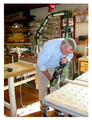
In these photos you can see the Domino machine with the saddle fences set for the 50mm width of the platform frame members and the fence set to center the Domino mortise on the 20mm thickness of those pieces.
