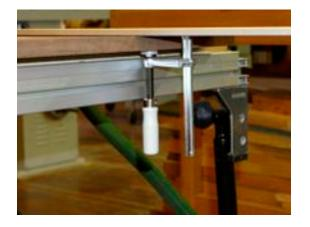
clamp a long Festool guide rail parallel with my intended line of cut for the sliding dovetail slots that will hold the side skirts (photo above).
