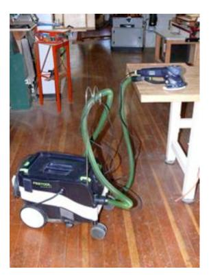
with all of the Festool sanders and cutting tools. Combined with the 9 hole vent pattern in the round pad sanders, and the variety of hole patterns in the other sanders, this potent team keeps the air around the sanding area much cleaner and safer for the person operating the sander.
