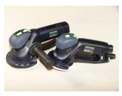
action. The green switch on the top makes the mode change. In one mode they act just like the ETS random orbit units. Switch modes on the RO 150 or the RO 125 and things get very different. The second mode on both machines is a hybrid between the gear driven pure rotary motion of the RAS 115 and the pure random orbit motion of the ETS units.
