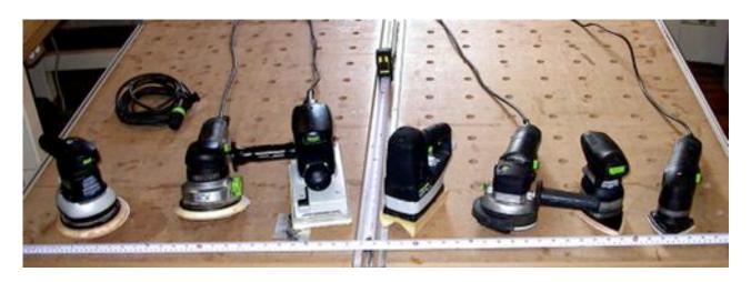
There are basically three different ways the abrasive can be moved by a machine sander: *linearly in a fore-aft motion, in a circle in a rotary motion, or back and forth in an arc.* Festool uses the first two motions but not the arc motion.
