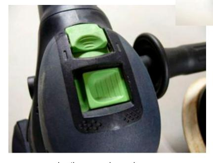
new version the same change is accomplished by simply moving the green rectangular button on the front top of the unit. Faster and far handier. The other green button shown is the on-off switch positioned to be on top right where your
