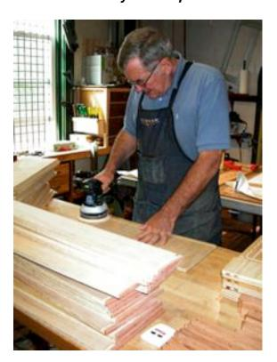
*in a random motion*. This produces very fine finishes with little or no scratching so long as you keep the pad flat on the work surface. Tip the pad to get more
