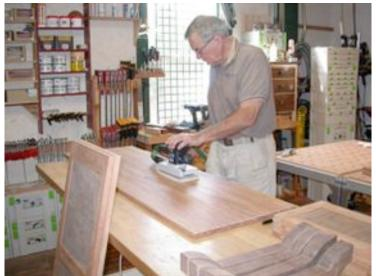
The **DX 93 E "Deltex"** sander is a specialty sander with a number of tricks up its small "sleeves." It rotates in a short orbit to prevent the scratches that I found
