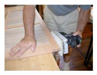
As pictured here you can see how the large flat surface is ideal for rail, style and panel components where a tip of the sander could well leave an undesirable depression along an edge.
