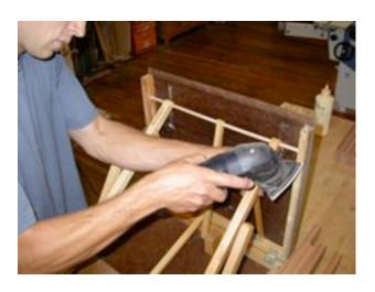
".... designed for strong abrasion through reduction gearing ..... ideal for stripping off old, thick and stubborn coatings," I find it also is one of the gentlest and most easily controlled of all the Festool sanders when the speed is turned down. I don't make scale models, but, if I did, this would be the first sander for which I'd reach.
