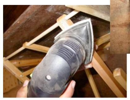
dust. Dust collection with the Festool supplied materials which do have the proper holes is excellent.
