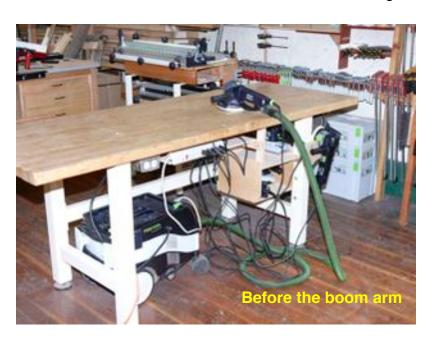
were plugged is gone, replaced by the one power cord that is right beside the vacuum hose. All the sanders are still in the same place and right at hand, it is just that now the hose and cord are both up off the floor and out of my way.
