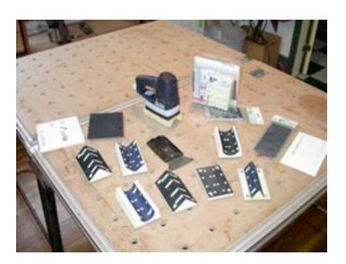
center of this photo) is offered as an accessory. Since the motion of the LS 130 is purely fore and aft you can use this to scrape off wallpaper, carpet, and other glued on materials far more easily than you could do by hand.
