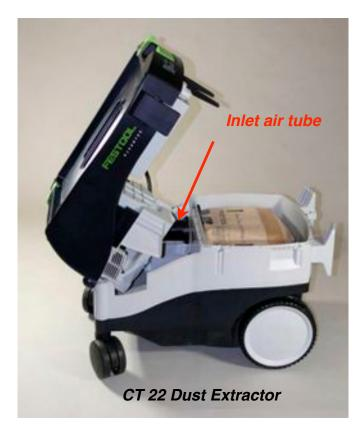
The CT 22 and larger units are different. First, the top hinges open rather than lifting off. The disposable bags fit into a chamber tightly connecting to the incoming air hose tube shown in the photos above and to the left.
