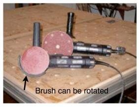
This is a VERY aggressive machine capable of removing a lot of material in a hurry. This much abrasive action generates a lot of heat. It takes a light touch to prevent digging the pad too far into the work piece and to prevent overheating of the pad or the work piece.
