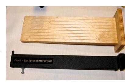
There are two black metal magnetically mounted **frame stand off laser target arms** included with your kit. Follow the instructions to mount these to the frame near the front and
