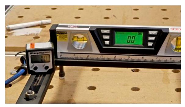
While I found the back lit Sears unit to be easier to read, it was also large enough to be awkward on my stand-off plates requiring the bungie holders to be mounted to the back of the vertical member where they were less effective in holding the stand-off plates securely to the rims as shown
