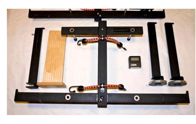
screws. The upper arm is free to pivot to make it easier to mount. The standoff pins are precision machined and come fully calibrated.
