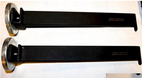
rear of the coach. The wooden laser target stands on the ground with one edge aligned to these arms for accurate reading of front and rear wheel parallelism.
