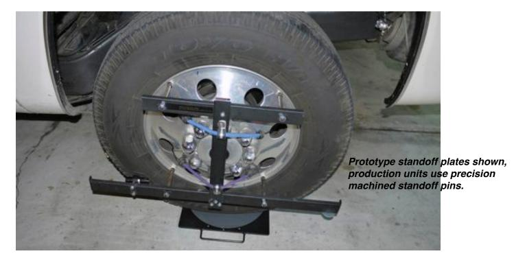
Place the now zeroed angle meter on top of the long arm and gently move the stand-off assembly to level the lower arm. That will also insure the upright member is exactly at 90 degrees to the parking pad surface.
