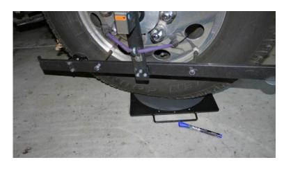
wheels have about the same caster angle somewhere between 2.5 and 5 degrees when the front wheels each have zero camber while pointing straight ahead.
