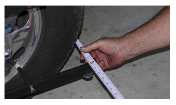
Ideally you will want to adjust the tie rods on both wheels by the same amount until the total toe is close to zero.
