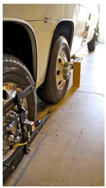
perpendicular to the wheel and zero it. Magnetically attach the angle meter to the vertical upright member and directly read camber. Record that reading.
