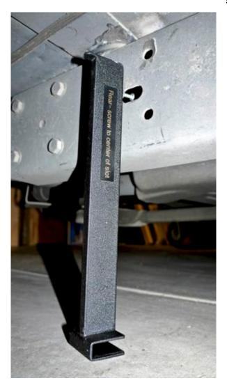
screw facing the slot in the frame behind the rear bogie. If the screw head fits inside the slot, you are at the factory recommended rear ride height. If it does not, add or subtract air in the passenger side air bag until it does.
