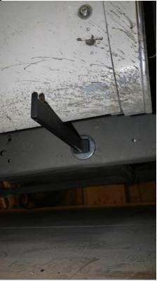
laser hits close to the same line on the target front and rear, your wheel is parallel with the frame. No need for great precision here. Close is good enough.
