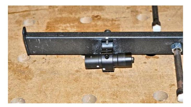
Once the beam was adjusted to be quite parallel to the mount, I put two white paint dots, one on the laser body and the other on the mount so the user can tell visually whether or not the laser has been knocked out of parallel.
